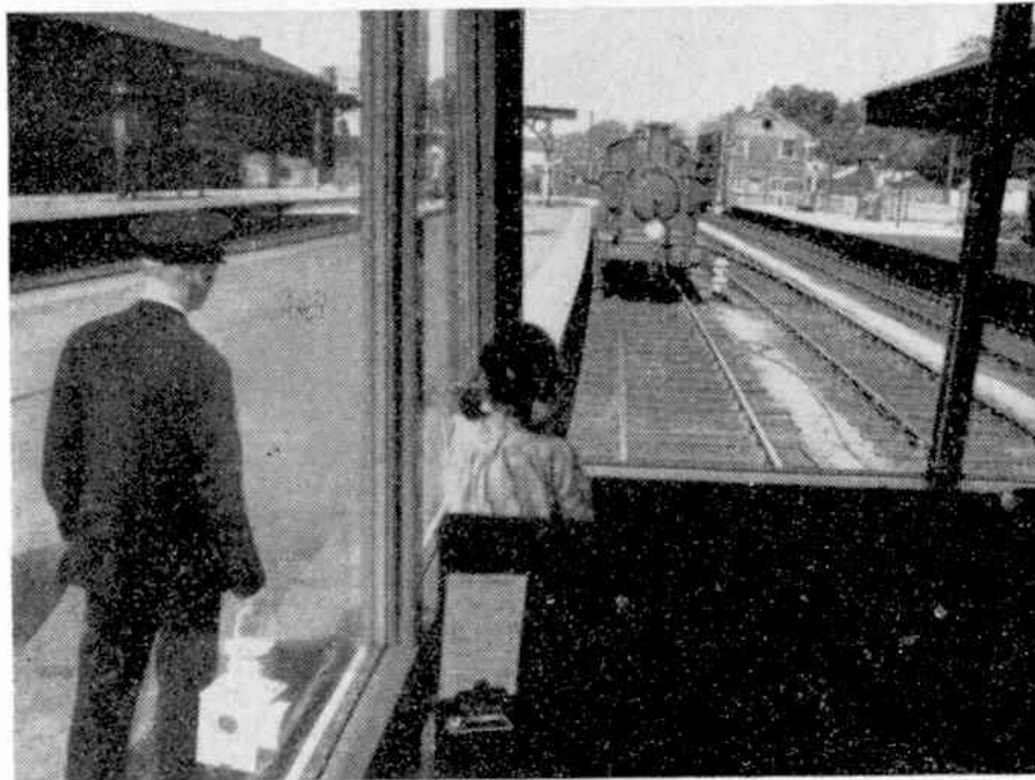
A banking engine approaches the rear of the up Devon Belle at Exeter St. Davids to assist the train up to Exeter Central. The guard has removed the tail lamp from the observation car, through the windows of which the photograph was obtained.
