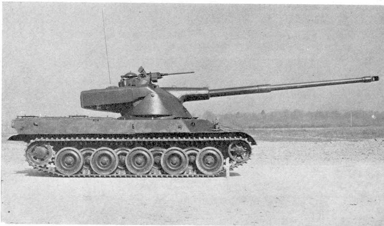
The fast, well armoured French Big Gun Tank of 1950, the AMX 50. Note however the very high silhouette, and the complicated turret with cramped interior.
