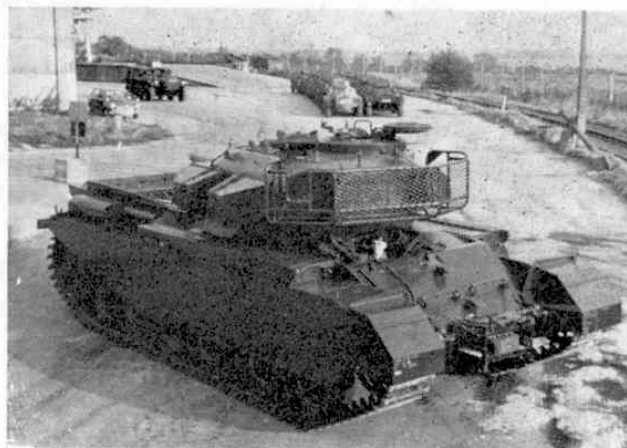
The very successful Bristol Centurion 9, designed in 1944/45. Modelled originally on the Russian "T34 concept" of a fairly fast general purpose tank having sloped armour and a big gun.
