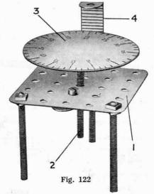
The model consists of a  $2\frac{1}{2}'' \times \frac{1}{2}''$  Flat Plate 1 supported on three legs composed of 2" Threaded Rods. Another 2" Threaded Rod 2 inserted in the tapped bore of a Threaded Crank carries on its upper end
