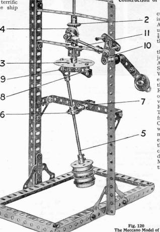
set-screws inserted in the collar are therefore provided with nuts that are locked against the sides of the collar to prevent the shanks of the screws touching the Rod 5. The latter is held in place in the Swivel Bearing by means of an ordinary collar and set screw.
