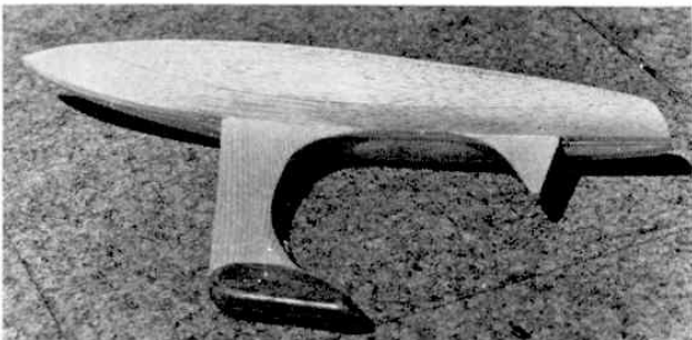
The hull and lead carved to shape ready for sealing and painting. It really is quite simple to carve and sand to the necessary shapes provided you don't rush it.
