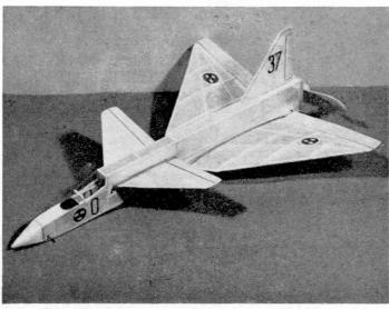
blocks of the correct height as indicated. Give elevator one coat of thin clear dope. Cut underfin from sheet, then dope and cement very firmly in place.
