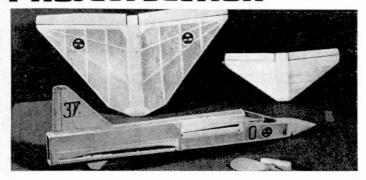
from both side and front views. Then carefully bend up the wing elevators about 3 in.
