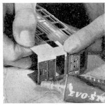
The rear entrance is enclosed by opaque plastic (Plastikard), cut to shape and glued into position using one of the popular impact adhesives, such as Evo-Stik or Bostik 1
