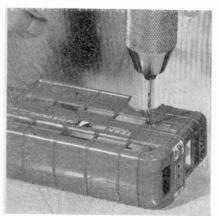
A new window is cut in the rear offside of the body by drilling a series of small holes in the casting around the edge of the proposed window and breaking out the surplus metal with a screwdriver
