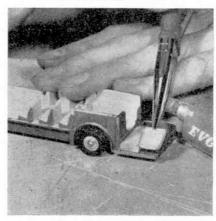
Once all alterations have been made to the chassis casting, the space previously occupied by the four front seats is covered by a sheet of Plastikard and the rear platform is built-up, with scraps of balsa wood to the level of the bottom step
