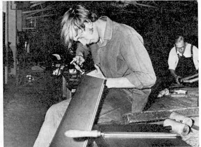
Shaping the bonnet of a Morgan is done by hand. A highly skilled and time consuming task.
