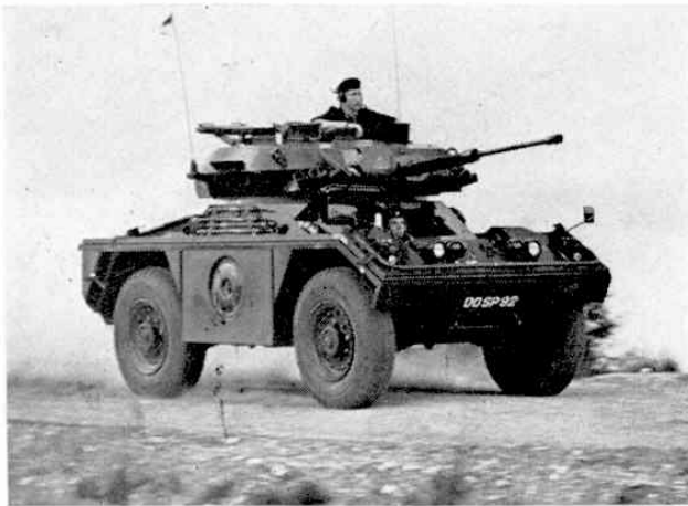
Britain's newest armoured car, Fox, small in size but big in performance, is quiet and unobtrusive but packs quite a wallop. Only 5½ tons, it is capable of well over 60 m.p.h.
