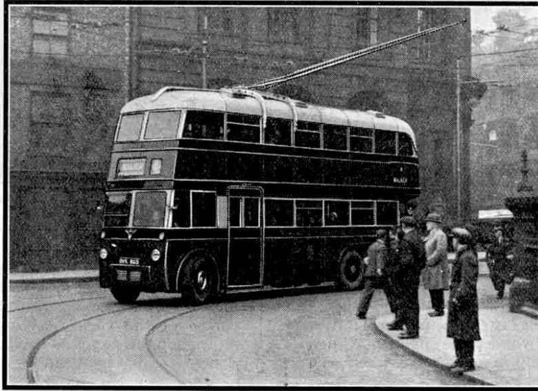
An A.E.C.-English Electric trolley bus with front exit, supplied to Newcastle Corporation Transport Department. This photograph and the upper one on the opposite page are reproduced by courtesy of The Associated Equipment Co. Ltd., Southall.
