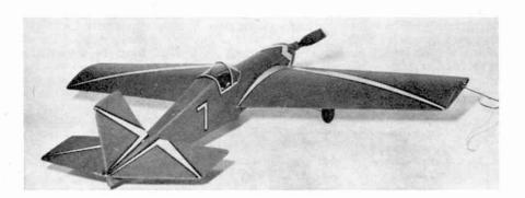
Pictures on this page show the original model. Only difference, apart from the colour scheme, is the cabin construction, made up of two pieces of acetate instead of one single wrap-round piece. If you prefer it, simply cut the top rear \$\frac{1}{2}\$ in. panel off at the back of the cockpit and fit the overhead acetate first. Leave to dry before adding the front screen.
