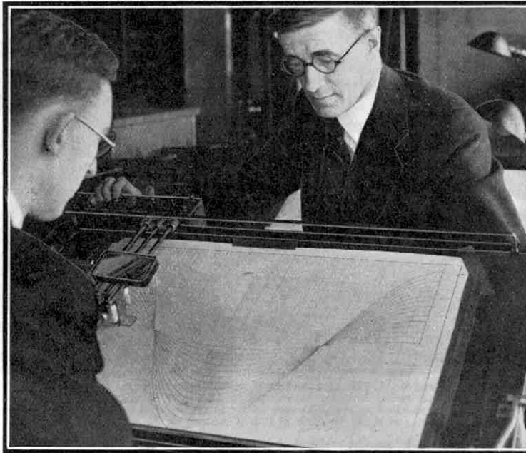
Dr. V. Bush of the Massachusetts Institute of Technology, Cambridge, U.S.A., watching the operation of the Differential Analyser, a wonderful machine he has designed for speedily solving intricate mathematical problems. A working reproduction of this machine in Meccano is described in the article on page 442 of this issue.
