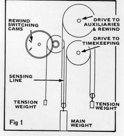
no way of getting more than two drives from one falling weight by cords and pulleys alone without an inordinate waste of height.
