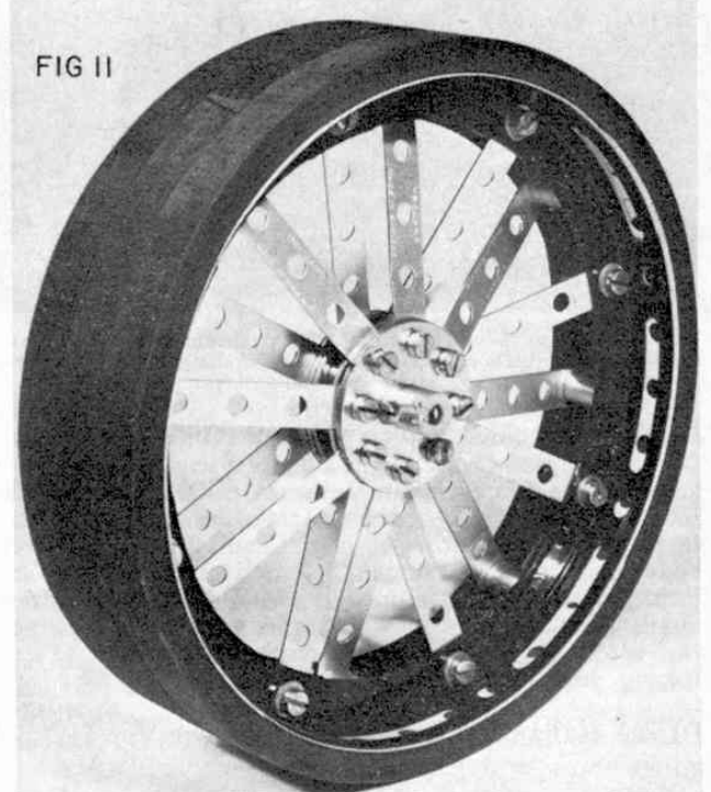
Fig. 11: A completed 16-spoke dished wheel for a Showman's Road Locomotive. The outer rim of the wheel is made from 5½ × 1½ in. Flexible or Plastic Plates trapped by rubber tyres or bands.
