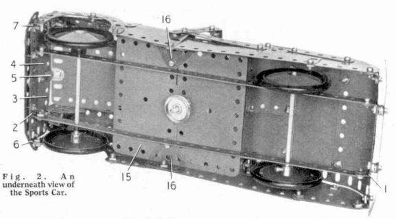
The floor of the car is a Hinged Flat Plate 15 bolted to two Trunnions 16 that in turn are attached to the side plates of the body.
