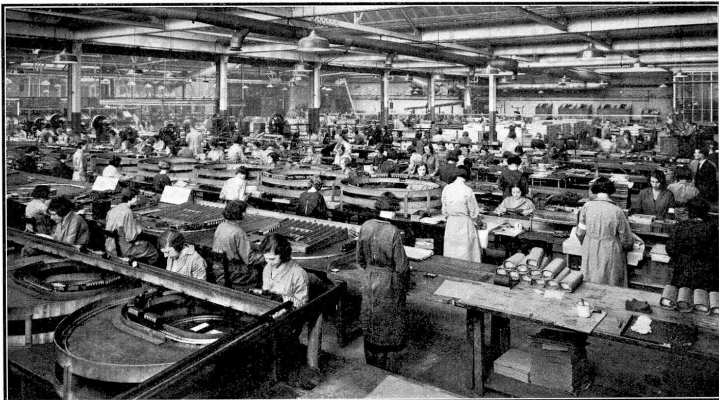
This illustration gives a comprehensive view of the Train Room with the locomotive test tracks a prominent feature in the foreground. The long conveyors used in the assembly of clockwork motors and for hand finishing can be seen in the background.
