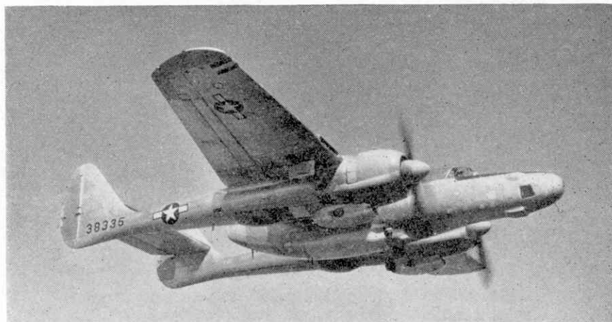
Production version of the 'Reporter' with engine supercharger intakes and underwing pylons for long-range fuel tanks. Our conversion (overleaf) was based on the modified, unsupercharged P-61A
