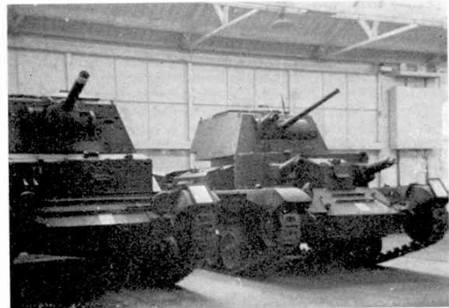
The Bristol Cruiser Tanks (left, A10; right, A9). Both are based upon the inter-war period Vickers designs, surviving in service until 1941. Note sub-turrets on the A9. These were a popular feature on many nations' tanks before 1939. War experience showed them to be excessively vulnerable, and some units used them as storage space. These tanks were said to "bounce like a pea on a drum".
