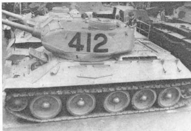
A Russian T34/85 of 1943. This tank was ahead of its contemporaries in having a larger cannon; a diesel engine; very simple construction layout and a very low ground pressure.
