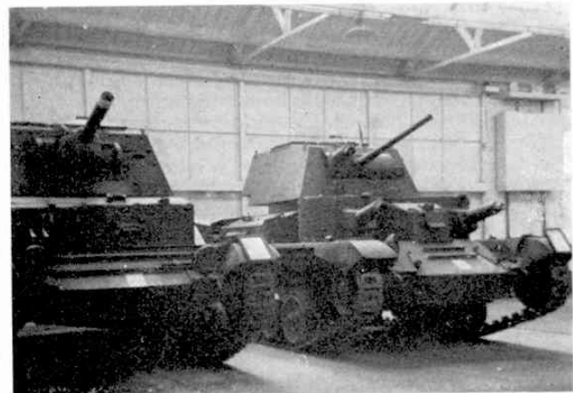
The Bristol Cruiser Tanks (left, A10; right, A9). Both are based upon the inter-war period Vickers designs, surviving in service until 1941. Note sub-turrets on the A9. These were a popular feature on many nations' tanks before 1939. War experience showed them to be excessively vulnerable, and some units used them as storage space. These tanks were said to "bounce like a pea on a drum".
