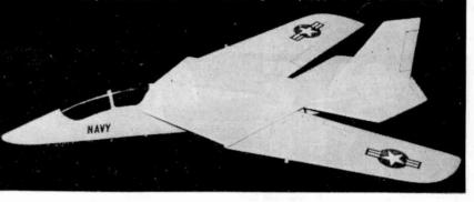
HERE'S SOMETHING different in catapult gliders -a swing-wing model on which you can set the wings at six different sweep positions and check the effect on performance. It's quite easy to make, but the method of mounting the wing panels on a pivot pin (short length of 16 in. dowel) is unusual, so study the plan, photograph and instructions carefully.
