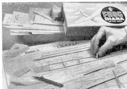
Here the fuselage is being built from strip balsa over the plan. Notice the greaseproof paper to prevent the parts from sticking to the plan
