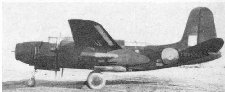
Above: the flat nose and matt black colour scheme distinguishes this Turbinlite-fitted machine, which is the subject of Ian Stair's scale plan on page 24. Below right: this is what it looked like from the pilot's seat
