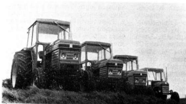
A line-up of Leyland tractors, models 384, 344, 253, & 154, with b.h.p. of 70, 55, 47, & 25 respectively.
