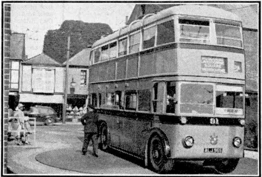
A Bournemouth Corporation trolleybus on the turntable at the Christchurch terminus. The use of a simple turntable avoids the need for a large turning circle equipped with overhead wiring.
