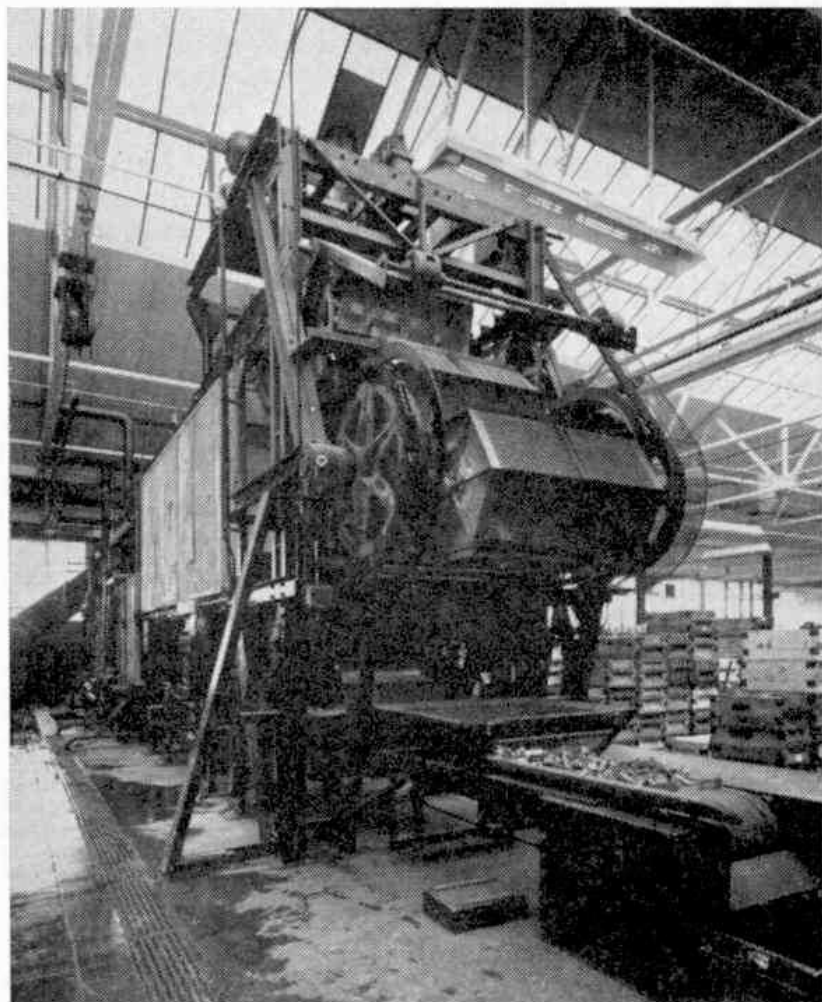
The delivery end of the Bonderising plant. Dinky Toys that have been Bonderised can be seen on the conveyor belt in the right foreground.
