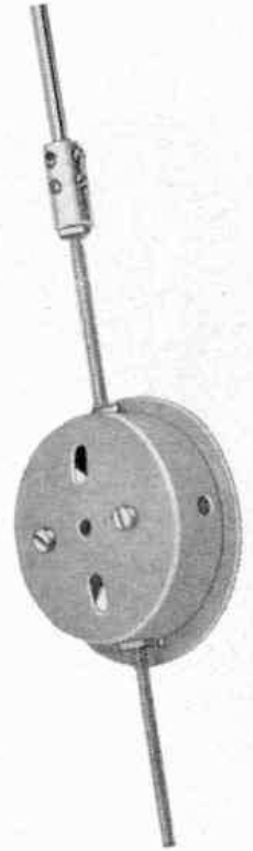
Fig. 2. The Clock pendulum and weight "bob".
