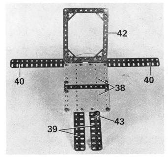
The drawing table included in the Easter Meccanograph, designed by Mr. Andreas Konkoly of Budapest, Hungary and featured in full constructional detail in this article. Unlike a drawing table on a traditional Meccanograph, which normally spins round, this unit slowly slews without revolving, tracing an elipse shape - hence eggpatterns for Easter!
