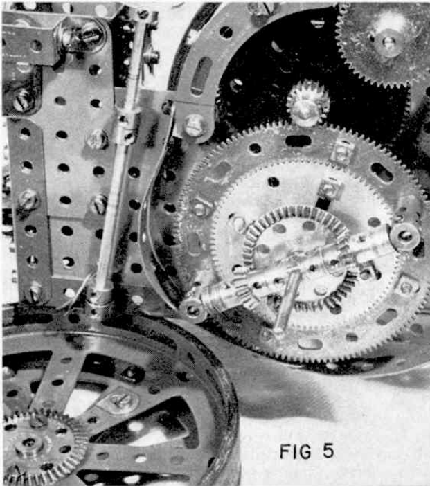
Fig. 5: The all-important differential gear which allows the traction engine to steer and perform winch operations.
