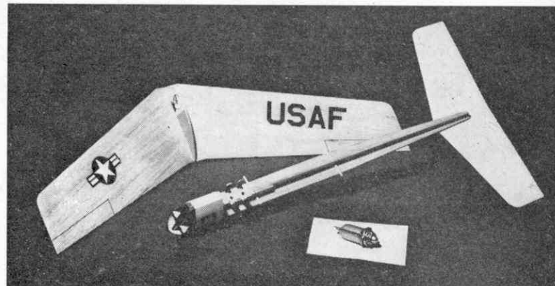
These photos show the parts of the model and the Jetex 50 unit with its clip mounting screwed in position
