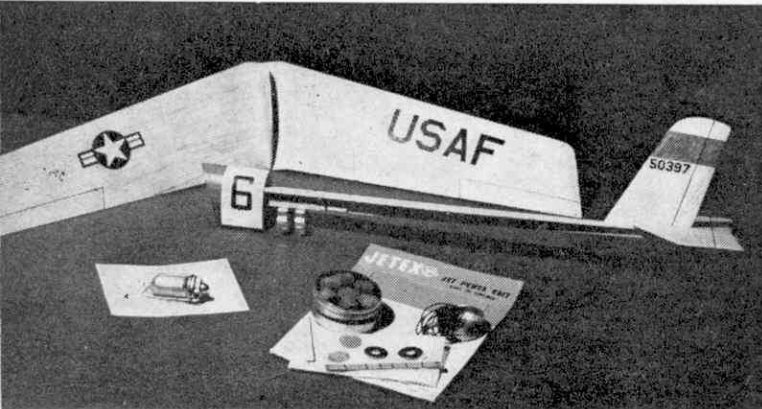
These photos show the parts of the model and the Jetex 50 unit with its clip mounting screwed in position
