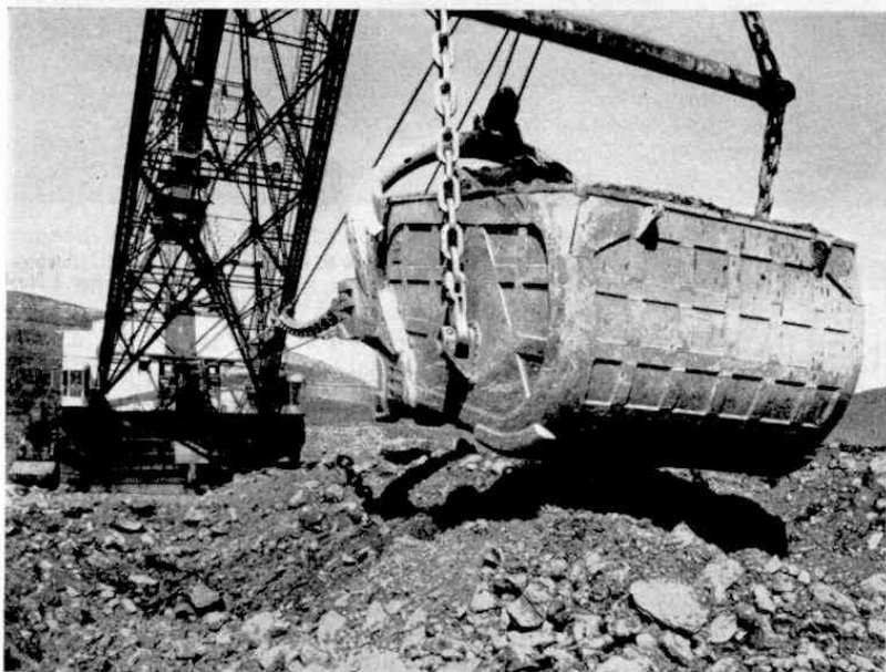
A close-up of the dragline's 40 cubic yard bucket which was manufactured by Hadfields, Ltd., of Sheffield.
