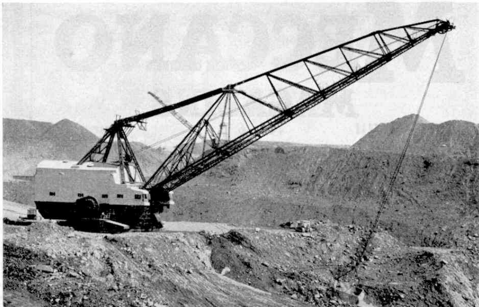
A general view of the Rapier W1800 Walking Dragline. All the illustrations to this article appear by courtesy of Ransomes and Rapier, Ltd.
