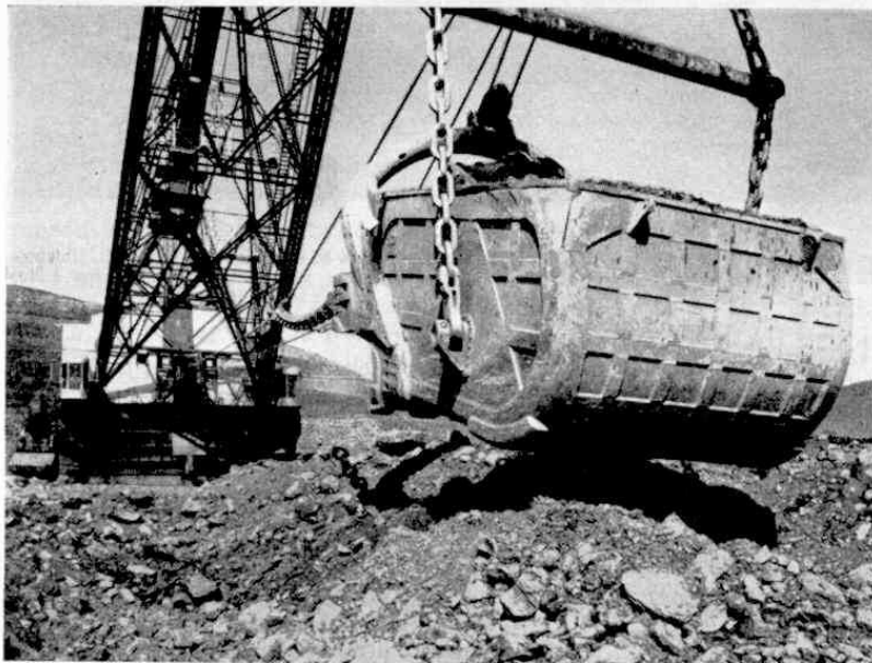
A close-up of the dragline's 40 cubic yard bucket which was manufactured by Hadfields, Ltd., of Sheffield.
