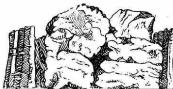
Fig. 1. Method of Constructing Early Breakwater*
