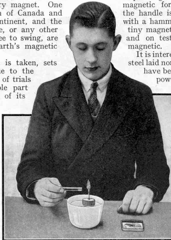
Fig. 1. A noating battery, the current from which flows through a coil of wire mounted above it.
