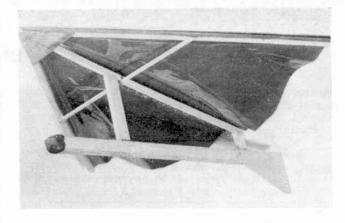
cept for cutting the fin from 16 sheet balsa and cementing to one side at the rear, as shown.
