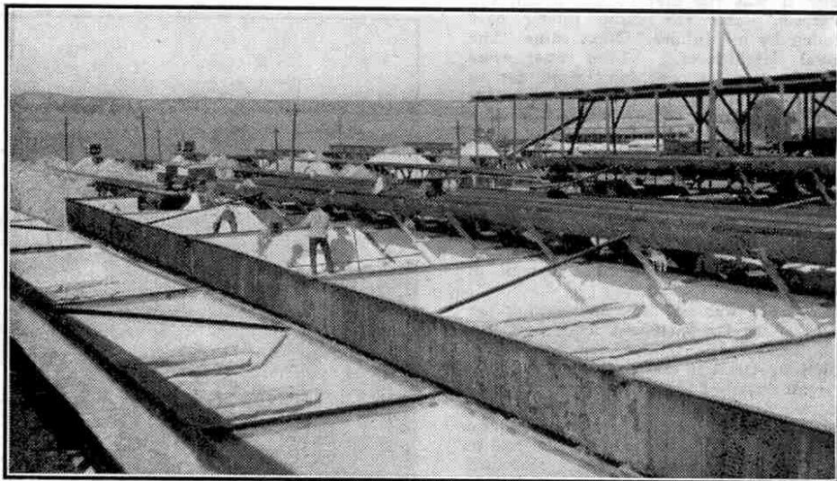
Making preparations to remove Chilean nitrate from the tanks in which it is crystallised. The illustrations to this article are reproduced by courtesy of the Nitrate Corporation of Chile Ltd., London.
