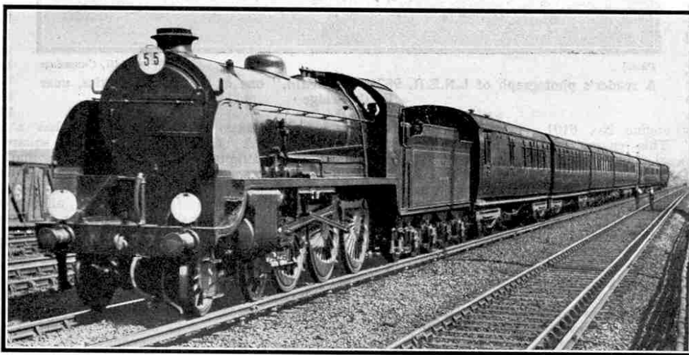
E.777 "Sir Lamiel" on the "down" "Bournemouth Limited," passing Durnsford Road Power Station. The locomotive is fitted with smoke-box deflectors in order to carry the exhaust steam clear of the cab windows
