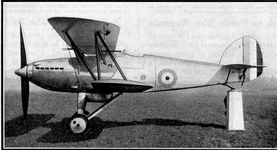
The "Kestrel"-engined Hawker "Fury" single-seater interceptor machine. This photograph is reproduced by permission of the H. G. Hawker Engineering Co. Ltd.
