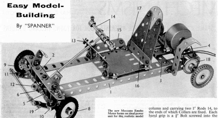
IN view of the popularity of Karting in this country today a typical Kart has been chosen as the subject for our simple new model Couplings and on this a 1" Pulley with boss fitted with Tyre is placed. The Pulley is free on the Rod and is held in position by a Collar 8.
