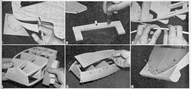
powered model the transom does not have a cutout—see Plan A. These are then cemented in place on to the keel, as shown in Fig. 4, noting particularly the angle of the transom (5).
