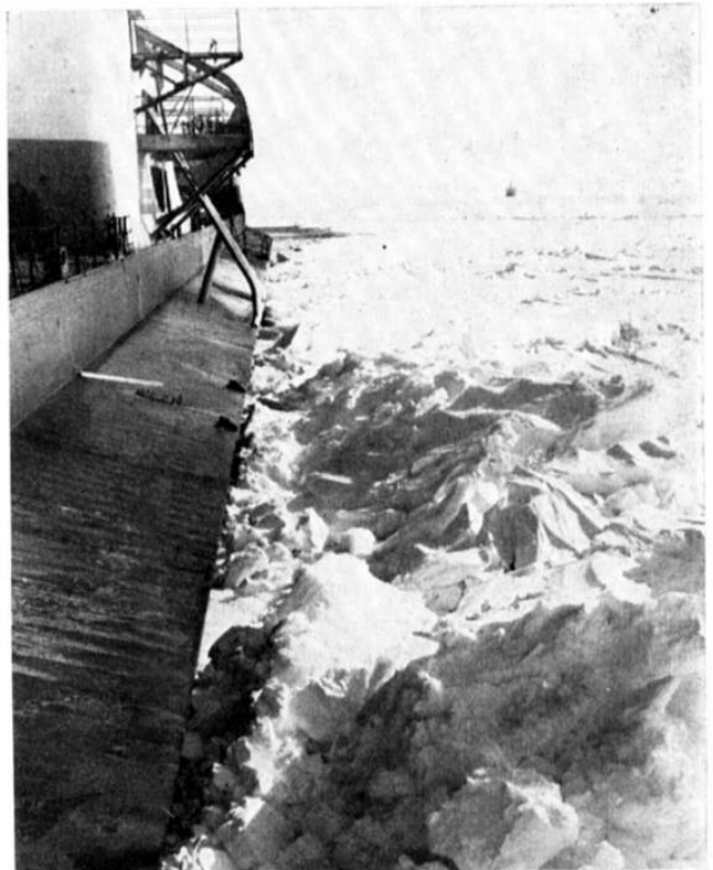
Right, The Manhattan trapped in heavy ridging ice in a northern area of Baffin Bay. Beyond is the new Canadian Coastguard icebreaker Louis S. St-Laurent which later moved in along the tanker to ease pressure and allow the ship to move again.
