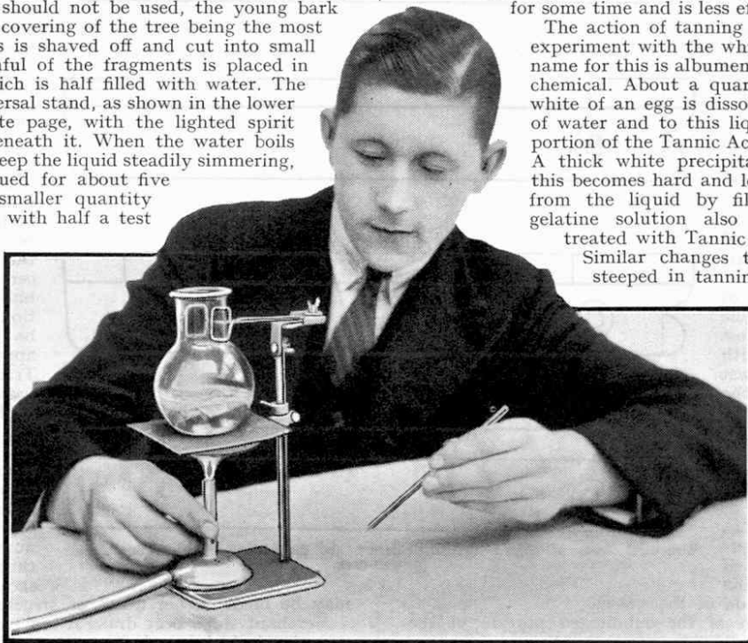
Boiling a strip of silk in logwood extract in order to dye it black. The silk has previously been treated with chemicals to enable the dye to be applied effectively.
