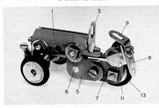
2 or 3, as the case might be. Note that the front Fishplate 2 points vertically downwards, while that at the rear points vertically upwards to represent the windscreen.
