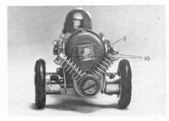
"spider" from a Universal Coupling, in adjacent holes of which are screwed two ½ in. Bolts 10, each carrying a Compression Spring on its shank. These Bolts, with their Springs, represent the engine cylinders, an exhaust pipe subsequently being represented by a Centre Fork 11, held in Rod and Strip Connector 6.
