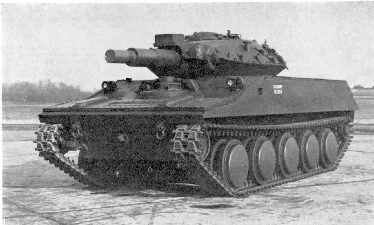
U.S. Airborne Tank M551 "Sheridan"—note riveted construction.
