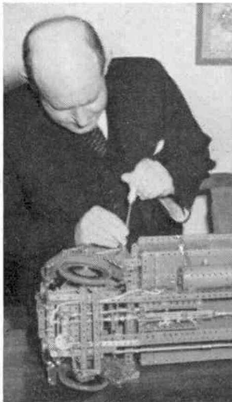
Fig. 4. Another view of the Albion Chieftain showing the details of the chassis.
