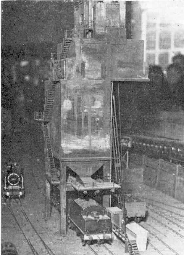
A true to scale Gauge "O" coal bunker on the West Lancashire layout. This model, built by R. C. Chown really works! The coal wagons are lifted up and the coal is then tipped into the waiting tender.
