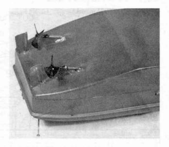
paint is not essential. Use flat grey paint for hull, deck, inside of bulwarks, ramp, etc., red oxide for hull below waterline, and white for superstructure.
