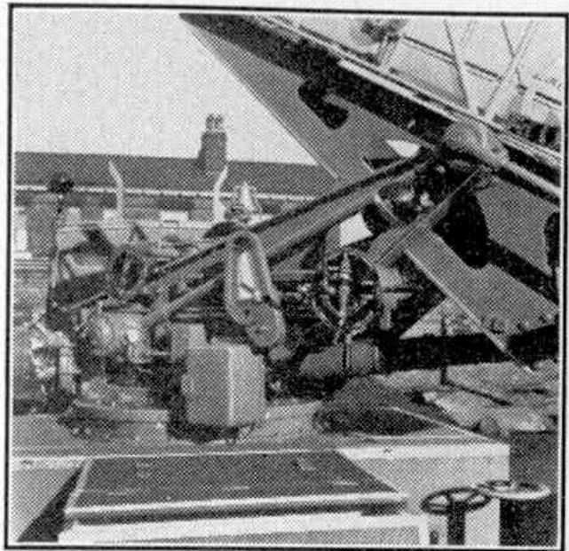
The operating controls of the Morris turntable fire escape ladder. In the centre is the special indicator that automatically stops operation when the ladder has been extended to its safety limit.
