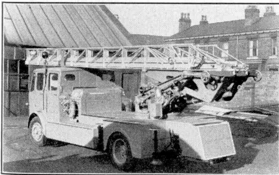
The new Morris fire escape on a Leyland Beaver chassis. Photographs by courtesy of Leyland Motors Limited.
