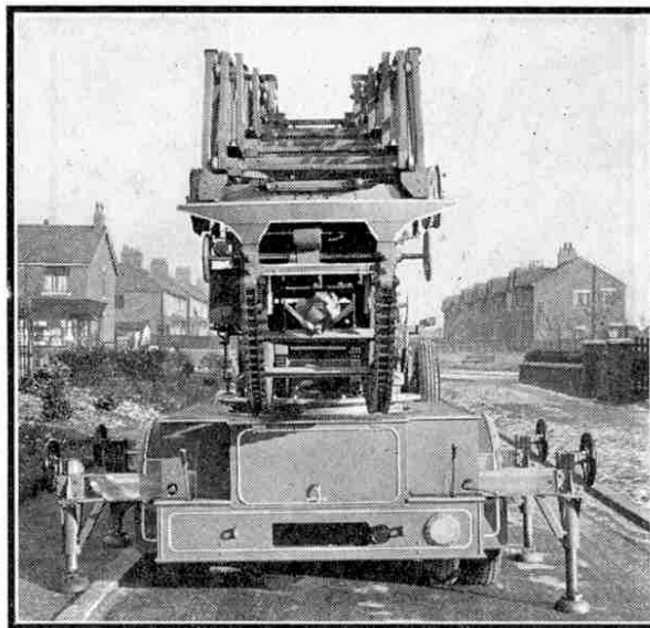
When the ladder is to be raised and extended, jacks on outriggers are lowered in order to give stability to the escape.
