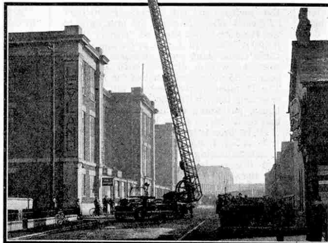
The ladder extended to its full length. It is in five sections with a total length of 132 ft., but similar escapes may have ladders up to 160 ft. long.
