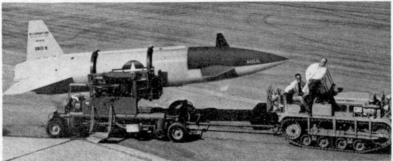
A Bell Rascal powered bomb is here shown secured to a ground-handling trolley for transport across the airfield.
