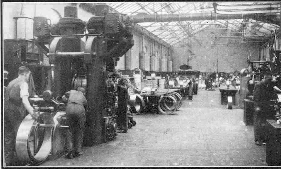
Fig. 3. Rolling stainless steel strip for aircraft manufacture.
